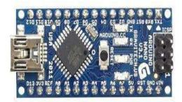
The Arduino Nano, as the name suggests is a compact, complete and bread-board friendly microcontroller board. The Nano board weighs around 7 grams with dimensions of 4.5 cms to 1.8 cms (L to B). This article discusses about the technical specs most importantly the pinout and functions of each and every pin in the Arduino Nano board.
